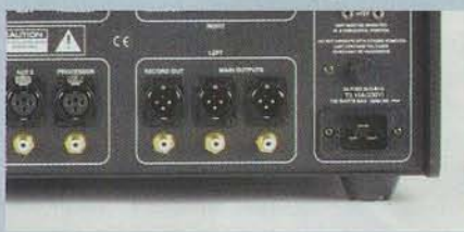
IEC mains inlet (left) requires large plug type
